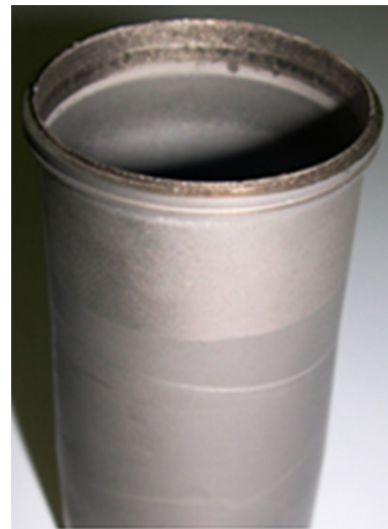
Figure 6.—SN18 test article: Condition of rejector-end flange after removal of permeometer flange using electric discharge machining.
